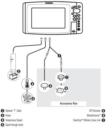
Inside the boat there is often a channel or conduit used for other wiring, this can be used to route cables. Be sure to route the cable as far as practical from the antenna cable of VHF radios or tachometer cables to reduce the possibility of interference. The GPS receiver cable should not be cut, and care should be used not to damage the cable insulation.
